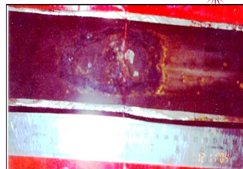
Fig. 1: Photograph showing the nature of corrosion attack. Deep corrosion pit is seen
